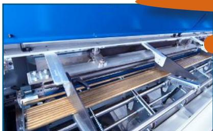
The **linear magazine** is formed by a single rack (260 mm) designed to load bars of diameters between **4** and **20 mm**.
