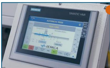
The **new one touch operator interface** can facilitate usage by less experienced operators and also has the ability to **store part programs** and easily recall them if needed. It is possible to remotely operate the bar feeder from the panel of the lathe\*.
