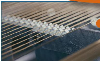
The bar **selection** system is very precise and allows selection with maximum reliability down to **2 mm bars**.
